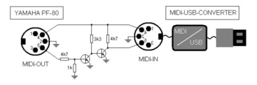
It took me some time to find out what was going wrong. One way (possibly the only one) to make a YAMAHA PF80 run over an USB connection is to connect it with a homebrew interface to a cheap MIDI USB Cable (note that ground connection must be accessible on both MIDI-connectors). <u>Arvydas</u> describes his modification at the same converter. Instead of some external parts he adds a missing opto-coupler inside the converter to meet the MIDI standards.
